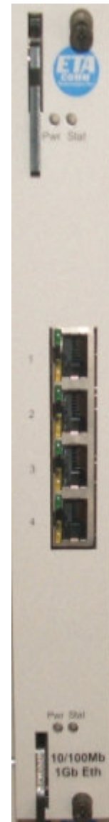
Figure RJ48C Interface
